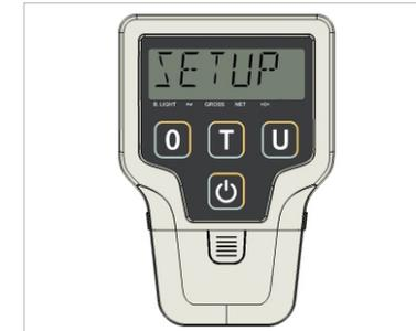
2. Press the "T" key to enter the setup mode
