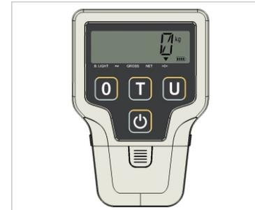
1. Press "U" key and "T" key simultaneously for Setup mode in normal mode.
