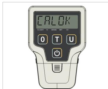
9. Calibration is deemed to be completed once "CALOK" is displayed on the screen.
