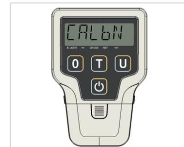
6. Make sure that there is no cargo on the frame, and Press "T" key to confirm calibration.
